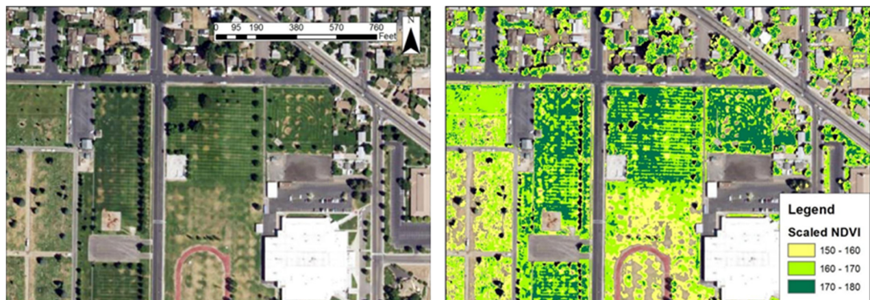
Figure 4. An example of determining the NDVI threshold value for irrigated areas. These images are for Study Area B with the true-color image on the left and the NDVI raster overlay on the right. In the NDVI image, yellow, light green, and dark green values indicate increasing levels of healthy vegetation, while no-data areas indicate non-vegetated landcover.
