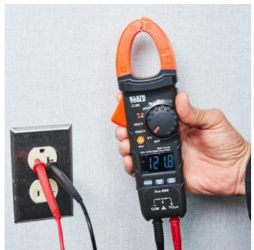
And a multi Meter that can read AC, DC, and Ohms of resistance. Can be auto ranging or not. Can be clamp meter or not. But consider this tool as the most important one you will be using while troubleshooting. So don't go cheap.
