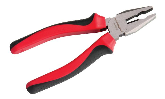
Blunt nose pliers. Important to be blunt nosed. Plays a big roll in the twist of the wire prior to the inclusion of the wire nut.
